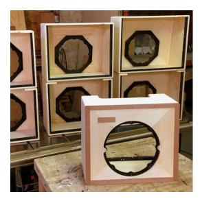
This cabinet design is quite different from traditional guitar speaker cabinets, which use a plywood baffle board attached to the cabinet with screws and wooden cleats. By comparison, the Sugarland's unified solid wood construction is significantly more difficult and time consuming to build, but the results are quite extraordinary – an example of impractical methods that help the Sugarland move beyond the performance of typical "boutique" amplifiers.
